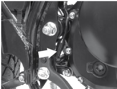
Rear brake light switch is located at the right side of chassis. Adjust the rear brake light switch as follows: Lift or lower the switch, so that, when the brake pedal is pressed, the lamp is lit before feeling a pressure.
