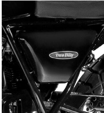
The tools box is right of side cover. To open the box, insert the ignition key and turn it clockwise and take down the box cover.
