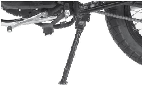
The vehicle is equipped with a side stand .
