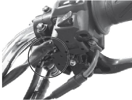
The front brake light switch is located below the brake lever. Loosen the screw and move the switch position back and forth to find the point where the lamp is lit immediately when pressure is applied but before the lever is fully pressed.
