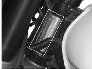
The Chassis number (or VIN code) and engine number are necessary for registration of your motorcycle. The numbers are also needed when ordering components or spare parts.
