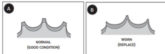
*Note\*: If worn, the pinion, crown and chain have to be replaced; using a new chain with a worn pinion or crown, the chain will rapidly wear out*
