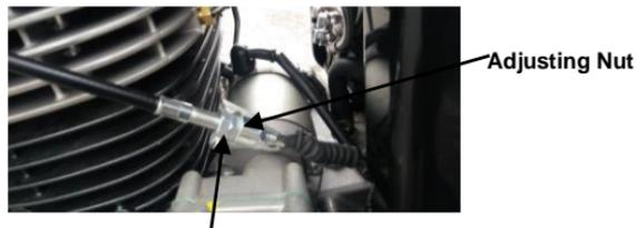
Remove the clutch control line on the handle end, and then remove the clutch operating arm on the engine end; turn the clutch operating arm by a proper angle and remount it, and then mount the clutch control line, finally adjust it to a satisfied free stroke according to the fine adjustment.
