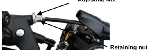
If a satisfactory free stroke can't be achieved by fine adjustment, remove the clutch control line on the handle end to adjust the engine end.
