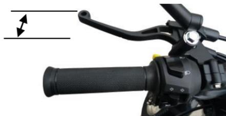
The clutch is adjusted by stretching the cable using the adjusting unit positioned on the handlebar.
