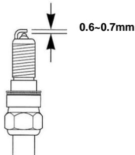
Carefully remove any accumulated carbon and contaminants with a spark plug cleaner or soft wire brush. Ensure the spark plug washer is in good condition.
